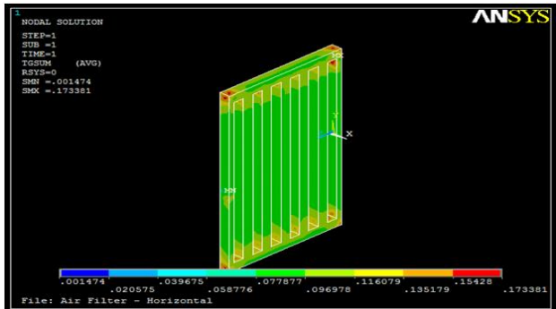
Fig 7.9: Temperature Gradient of AIR FILTER – HORIZONTAL
